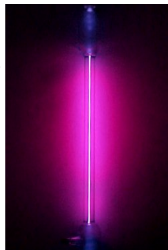
(Above) The inner working of a spectroscope and a gas discharge tube. (Below) A common spectroscope (Right) A Hydrogen discharge tube
