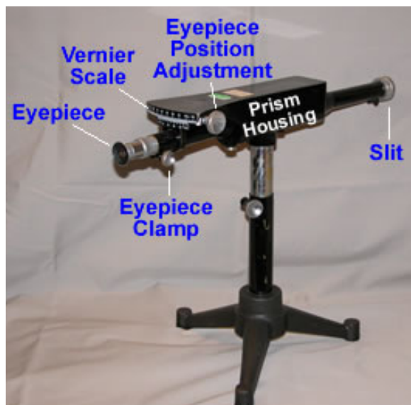
(Left) A Spectroscope. Light enters the slit and goes through the prism housing (may be replaced prism with a diffraction grating). The observer uses the eyepiece to see the image.
