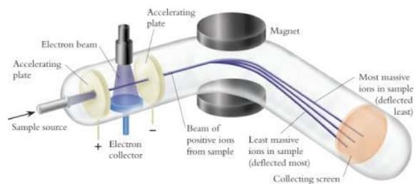
Schematic representation of one type of mass spectrometer. An electron beam fragments gas atoms or molecules into positively charged ions. The ions are accelerated and then deflected by a magnet. More massive particles are deflected by smaller amounts than less massive particles.
